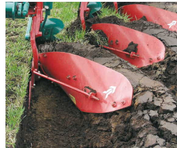
furrow profile body No. 28 working depth: 26 cm, bottom: 30 cm, width 73 cm
